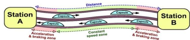
Figure 1: The conceptual Hyperloop diagram. (Nøland, 2021)
