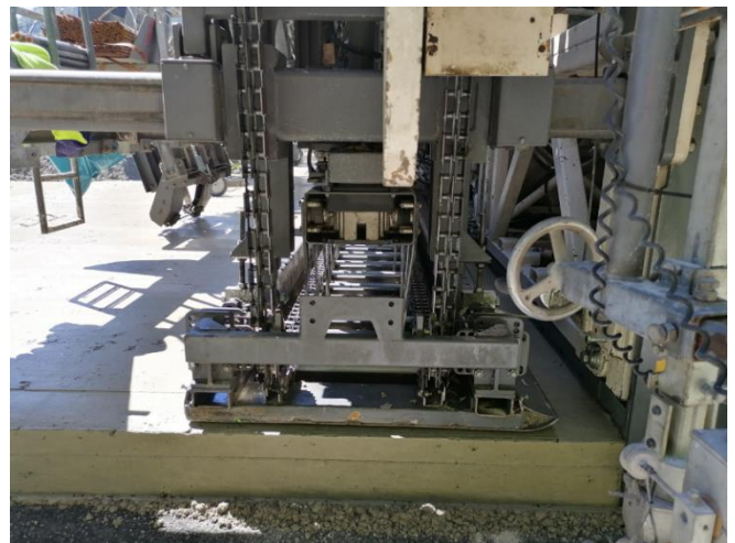
Figure 22. Vibrator for under-concrete; standing edge for concrete with high green strength, Source: K. Hrapović, 2021
