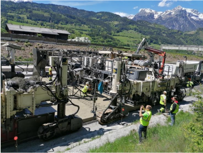
Figure 11. Concrete paver with even 12 crawler tracks for paving bottom and top concrete – front part, Source: K. Hrapović, 2021
