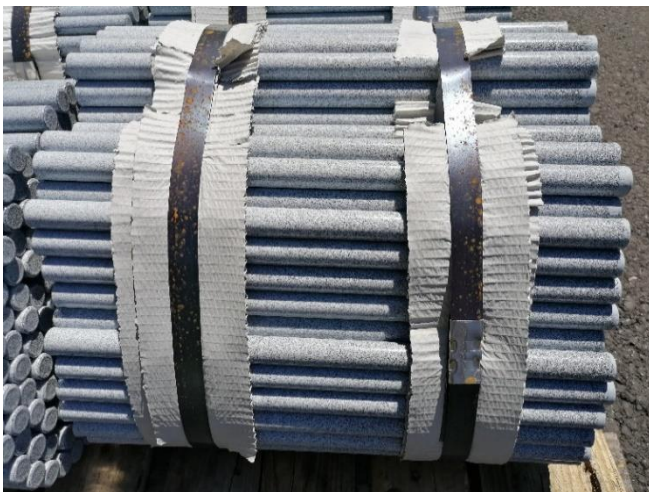
Figure 4. Smooth round steel dowel, Source: K. Hrapović, 2021
