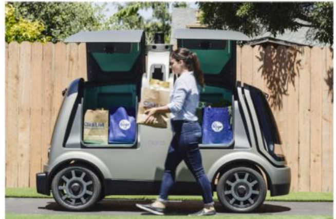
Figure 3. An example of Nuro ADV for last-mile delivery Source: https://nuro.ai/ . (Accessed 22 November 2023).
