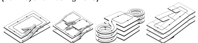
Figure 4. Ramp systems: a) Full ramps, b) Half ramps, c) Spiral ramps, d) Parking ramps Source: FGSV 2005
