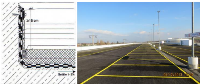
Figure 14. Pavement structure exposed to weathering with 3.5 cm mastic asphalt layer chipped on a 3 cm protective or intermediate layer Source: Felsing & Piring 2016a
