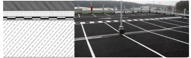
Figure 16. Pavement structures exposed to weathering with asphalt concrete wearing course with 3 cm AC 8 deck on a 2 cm protection layer on a 2 - layer bituminous sealing Source: Felsing & Piring 2016a
