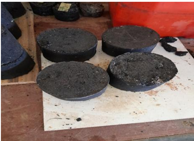
Figure 1. Asphalt Concrete with Waste PET Plastics Bitumen Modified
