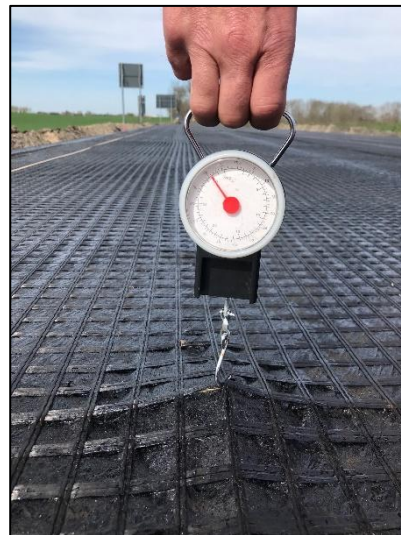
Slika 5. HOOK test Source: Jens Baumann
